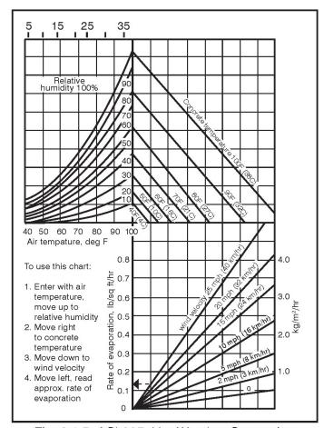
Fig. 2.1.5, ACI 305, Hot Weather Concreting
