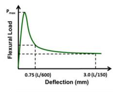
Schematics of a typical C1609 test result
